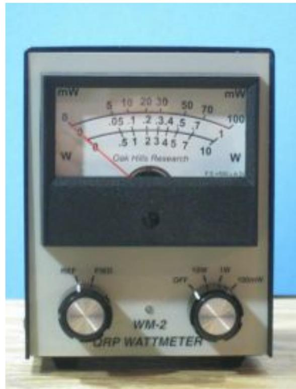
The WM-2 has three power ranges of 100mW, 1W, or 10W with a claimed accuracy of 5% of full scale. It is powered from either an internal 9V battery or an external power supply. The meter measures both forward and reflected power so you can use the readings that you make to calculate SWR if you wish.
