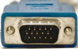
Here is your VGA connector as seen on the cable that was attached to the back of your old computer. It has 15 pins. The cable may be missing one or more unused pins, but all 15-pin sockets are present in the connector on the back plate of your computer.
