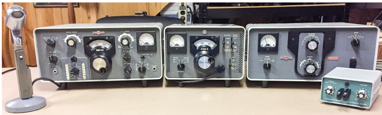
Collins KWM-2A Transceiver, 312B-5 External VFO, 30L-1 Linear Amplifier Also, Electro Voice 638 Microphone and Heathkit HD-1410 Keyer
