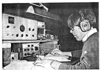
HUGH PUTNAM K9ZUB, Mequon, operating a code set up. The box at the upper left is a home made transmitter electronicly coupled to the receiver below it. When a signal is heard on the receiver, the transmitter is ready to go on the same frequency as the received signal.
