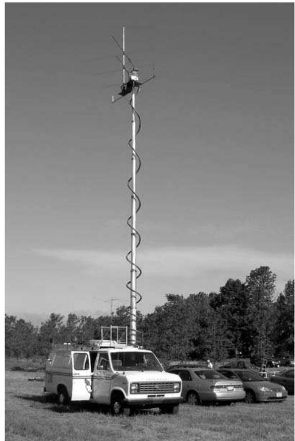
**The most easily raised tower was that of the OZARES communications van. Only the push of a button was required to get the camera and the UHF and 6 meter antenna raised.**
