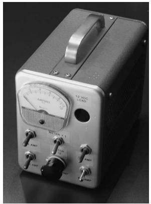
The completed 12 VDC Resistive Load Box.
