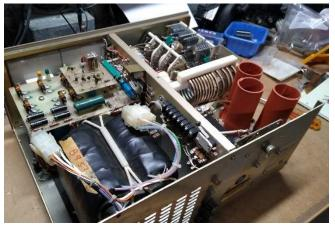
Last month I mentioned that I was working on an Alpha 78 linear amplifier. This amp sat unused for many years. I started with checking the filter caps in the high voltage supply. Everything tested good and the power supply came up with no problems. This amp has a modular design which allows the power supply and control board to be unplugged for servicing. A minor repair was needed in the power on timer circuit. I put the amp through its paces and got good power
