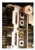
Notice in this closer view that the brass clip – that was the original compression trimmer – has been removed in the process of adding the new trimmer. The trimmer was supplied by Hallicrafters to customers.
