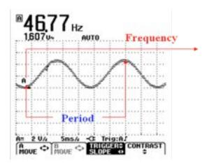
At the left is a snapshot of a scope screen displaying an AC voltage of 1.607V at a frequency of 46.77 Hz. We know this
