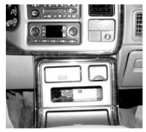
While the DVD compartment was also too small for the control head it did allow for rear access of the control head cable and fabrication of an "insert mount" for the control head.
