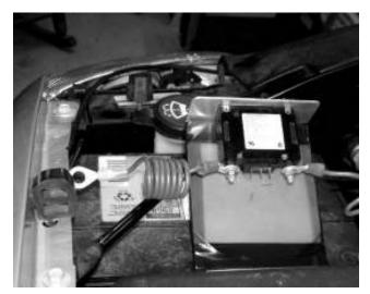
Here is shown the unconnected circuit breaker mounted in the aluminum bracket. The bracket was insulated with thick electrical tape in the area that inserts down along the side of the battery.
