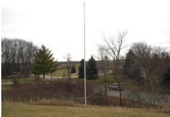
The loop size is a compromise between fitting in a reasonable space and good signal reception. A single support 25' tall does the job holding the loops up. The wires fit in a 30' diameter circle.
