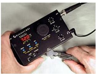
The Elecraft KX1 – a two band QRP transceiver with a keyer- receives SSB/CW & transmits CW only
