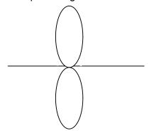
Figure 3 – Extended Zepp radiation pattern
