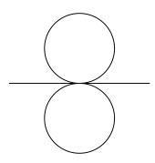
Figure 2 – Radiation pattern of a ½ wavelength dipole
