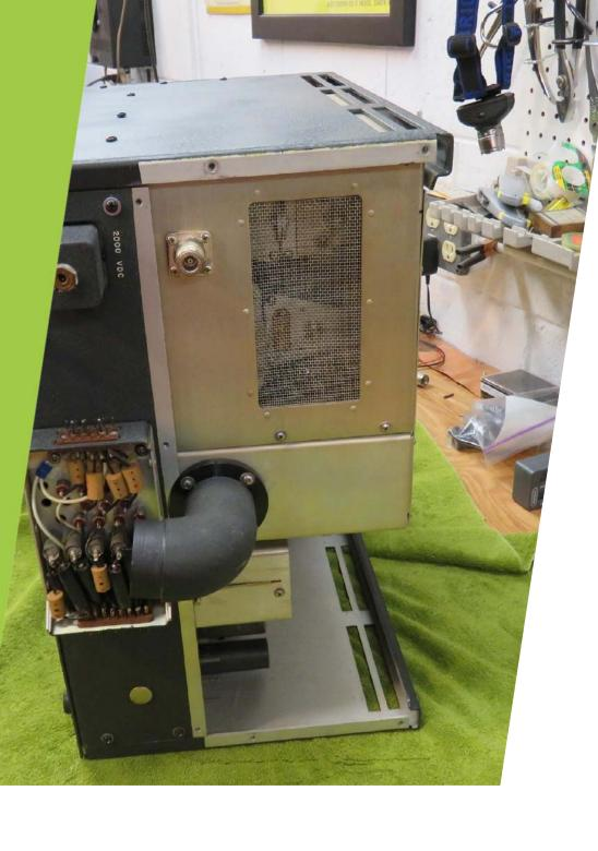
First the top cover and top back sheet metal was removed.
