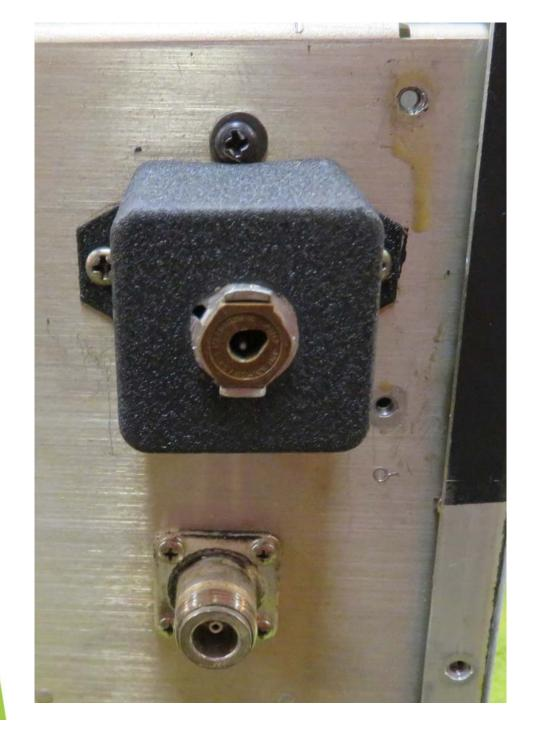
Now we have reached the point where we can actually start with the installation of the chassis mounted SHV connector.
