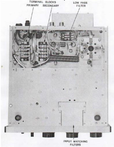
Again, the bottom of the picture is the front panel. The tube is at the top right. The power transformer connections are to the left of the tubes, along with the filament choke. The INPUT MATCHING FILTERS removable panel covers he input matching filter components. The ANTENNA CHANGEOVER RELAY (RLY-1) is between the tube sockets, The coaxial connectors for input and output are shown at the top right on the back panel. In that same area you can see the housing for the cooling fan.
