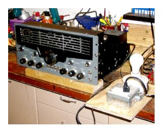
Once it is determined the suspect load has no short to chassis or other fault drawing high current the test switch can be turned "ON", shorting out the "dim lamp" and applying full voltage to the load being tested.
