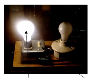
This "dim light" tester includes a switch across the "dim light" so that once the load is determined to not be "shorted" but operating normally the "dim light" can be "bypassed" in the circuit and full voltage applied to the load.
