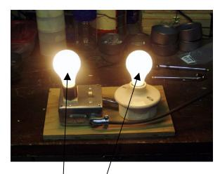
When the load (left hand bulb) is operating normally the test lamp in series with the load will glow dimly.
