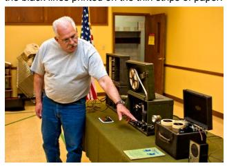
Yet another machine, much smaller than the first two, read a different kind of paper tape with short and long holes punched through it. A mechanical arm made contact through the holes and shorted terminals momentarily for the small holes and longer for the large holes! I had rigged up a little Code Oscillator with a light so the boys could see and hear the code being "read".
