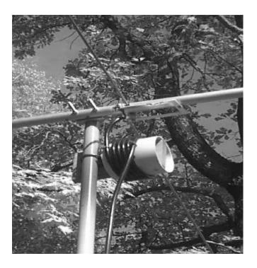
Balun of Coax Feeding a 6 Meter Beam Driven Element
