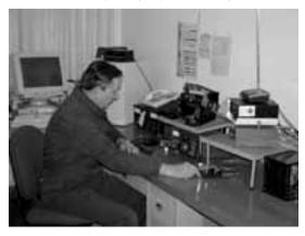
Eventually Leon progressed to the shack shown here which consists of an ICOM IC751A on HF feeding an Vectronics antenna tuner and either a TA33 beam or G5RV wire antenna for 160 through 10 meter operation. He runs an FT230 on 2 meter packet and an IC2000 on 146.97 etc. The FT730 in the background is monitoring the 443.75 repeater. Congratulations Leon, that's a real tidy shack.
