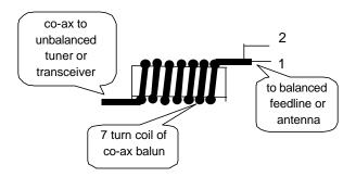
The co-ax balun can be simply a several turn coil of co-ax at the antenna feed point or it can be uniform coil of coax as wound on a PVC pipe. My preference is the uniform coils of co-ax wound on or within a PVC pipe as shown below.
