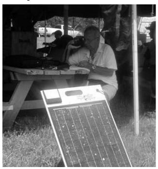
Hard to believe but with all that power and all those computers available, Ed Rate (AA9W) preferred to operate QRP at 5 watts with his new FT817 and the solar panel power source he designed and constructed. The solar panel puts out 14 volts at up to 3 amperes and was built from parts in Ed's junk box and Dayton. He made the
