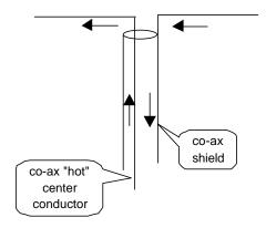
Under these perfect conditions the RF field created about the center conductor will be 180 degrees out of phase with that created by the return current along the inside of the shield and the two fields will cancel resulting in zero net radiation from the co-ax feedline.
