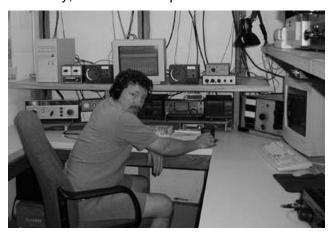
one of our more competative stations and operators, Fred Helmstetter (N9FH). His basic stations consists of an FT1000MP driving a TenTec Titan amplifier and an ICOM 746 driving a Henry Amplifier. Fred operates all the bands from 440 MHz through 160 meters and is a great contester.
