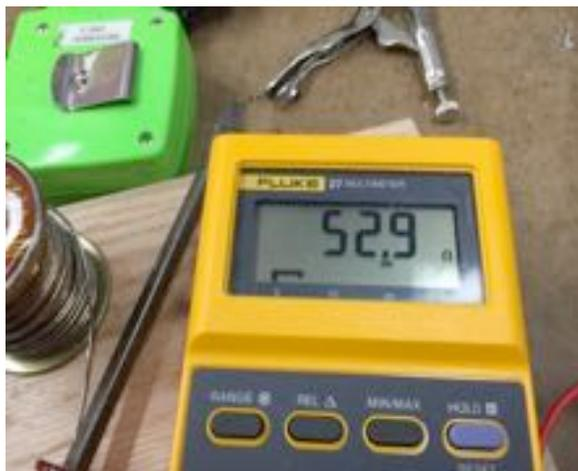
Next I checked the load resistance, four resistors in a series parallel connection. It looked fine. The last step was to mount the load to the cover and input connector, then check SWR using a MFJ-259B. (The item to look at is clamped in the vice.)
