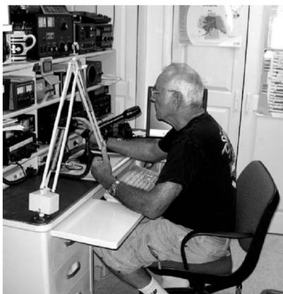
The "mic econo-arm" provides great arm and back relief during contesting and rag chewing while allowing free use of the hands to tune or manually log contacts. The mic is connected to the original mic desk stand via an 8 pin microphone extension cable I bought at Dayton and this allows continued use of the desk stand PTT switch and scanning ring.
