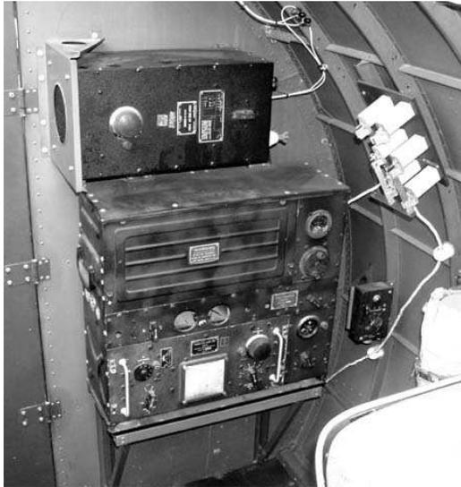
Behind the operator was the high power transmitter, the BC475. As I recall these were converted to run around 500 watts on the Ham bands. To change bands you replaced a complete tuning unit. These systems were not only some of the first high power Ham rigs following the war they came complete with a large case of TVI.
