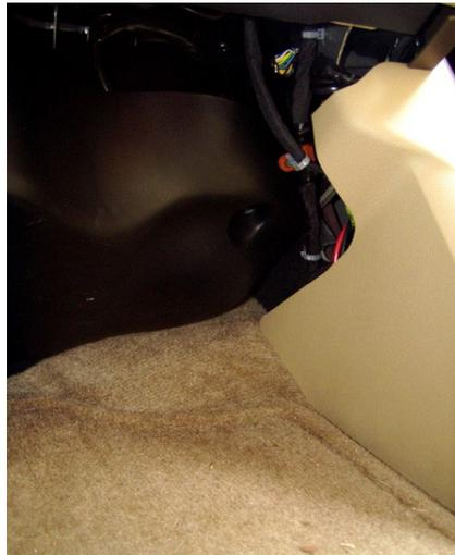
The wires were protected with plastic spiral and passed into the passenger compartment. From there they were passed behind the plastic side kick panel and then beneath the lower floor door moldings to the rear electronics. Problems solved except for the HF antenna.
