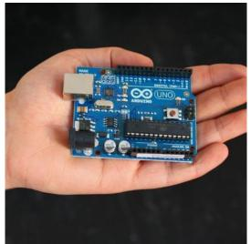
Arduino Uno microcontroller prototyping board. (photo courtesy Arduino: http://www.arduino.cc/)
