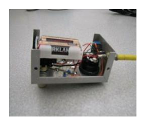
Photo (left) of the smaller of 2 wideband field strength meters built by Stan, WB9RQR. Photo (right) of the meter's construction.
