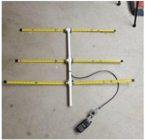
Fox hunting equipment: homebrew handheld yagi antenna and HT with attenuator attached.
