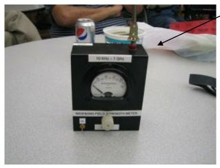
Photo of the larger of 2 wideband field strength meters built by Stan, WB9RQR.
