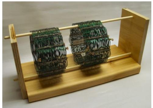
Fig. 3. L1 and L2 mounted on a cradle. Dowels through the openings in the windings allow the coils to slide. The dowels can be removed to allow taking the coils off the cradle for experimenting with different coils. The base of the cradle is 12 inches long.
