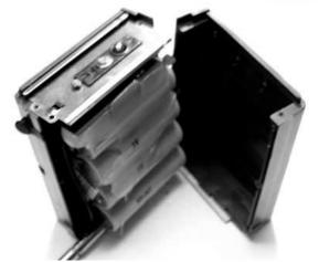
After unsoldering the original pack and installing the replacement pack (and temperature sensor) the case is easily reassembled.
