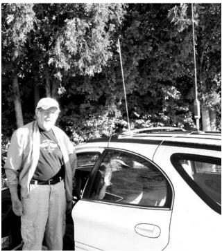
Tom is shown here with a unique approach to 40 meters mobil. The antenna is the loading coil and upper section of a 40-meter hustler antenna secured to the car with a magnetic mount. He claims it works good but I can't help but wonder about the SWR
