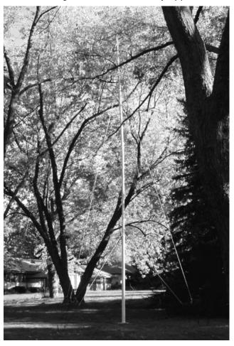
This is Mark's (KC9GST) newly designed 35 ft. Portable mast made of PVC pipe, a special surface mounting plate, 4 radial support pipes and quy ropes.
