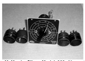
The McMurdo Silver Model 903 Absorption Wave Meter and 4 of the 6 coils used to indicate the frequency of the monitored RF field
