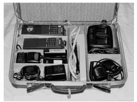
The case was divided into compartments with wood dividers glued and stapled into the case.
