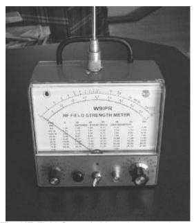
The HF Field Strength Meter is shown here with the antenna connected at the PL259 connector on top of the case. A 2-turn "sniffer" coil on a 3' peace of co-ax can be connected at the front panel BNC connector.
