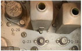
Note that all transistors not mounted to the chassis as a heat sink (Like Q-20 at the upper left corner of the picture to the left) were mounted in sockets (like Q-23 and Q-12 to the right). Today this presents problems with corrosion in so many unsoldered, low current, connections in the radio's signal path.
