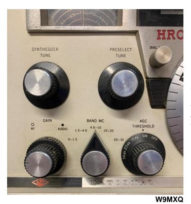
Note the "BAND MC" switch – lower center in this picture – lower lefthand corner of the Front Panel. In this example the selection is "4.0-10" – which includes the frequency we want to tune.
