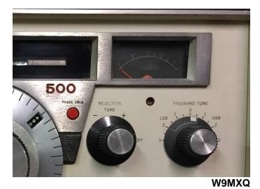
For reference – see this upper righthand quadrant of the HRO-500 Front Panel. This shows the location of the PASSBAND TUNE, and the REJEC-TION TUNE controls.
