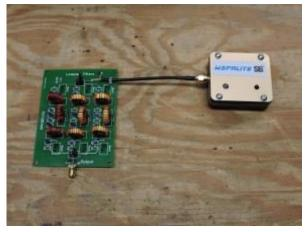
The device is called the WSPRlite (<a href="http://www.sotabeams.co.uk/wsprlite">http://www.sotabeams.co.uk/wsprlite</a>). It's a 200 mW WSPR transmitter that supports the 20m and 30m bands, and with the added Low Pass Filter kit it can operate on the 40m, 80m, and 160m bands. The WSPRlite transmitter comes assembled in a 2"x2"x0.75" enclosure. The only interfaces are a micro USB port for power and configuration, an SMA connector for an antenna, and a button to start transmitting.
