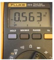
the suspect diode, first in one direction, and then the other. With the negative on the cathode there would be a needle deflection indicating forward bias of the diode and therefore conduction. Reversing the probes should indicate no conduction, i.e., a good diode. If there was conduction in both directions, the diode is shorted. That
