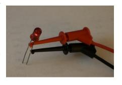
straight on and not off to the side as in the picture.) Again, the DMM will display the voltage it takes to forward bias and turn the LED on. In this case it is 1.63 volts which is enough to turn it on but not to full brightness which is usually around 2.2 volts.
