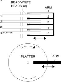
Sometimes the published drive specifications show it has one less head than it should (7 heads for four platters, for example). That is because one platter surface is sometimes set aside to hold head positioning data that the controller uses to move around the drive. So, the head is really there, but it is not usable by you to hold your data.
