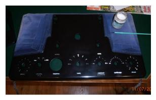
When repainting a panel it is a real challenge to match the paint color and to save the dial/knob markings that were silk screened on the panel.
