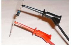
still holds true using a DMM except for one thing. In many cases, the DMM, because of the processor it uses, doesn't provide enough voltage to forward bias a diode while in Ohms. That is why there is a separate "Diode
