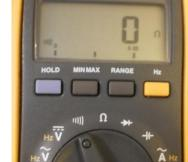
Check" you can do just that. You connect your test leads across the contacts you want to check; activate the relay, and <u>LISTEN</u> for a steady tone. When you release the relay, the tone should disappear. You may check this function of the DMM just by touching the probes together, or if you're
