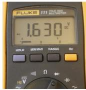
Can't remember if it is the long or short lead on an LED which is the cathode? Why not check it with the DMM? Just connect the test leads across the LED and see if it lights up. If not, reverse the leads and take note to the negative lead and the length of the LED lead it is connected to. (It will not be full brightness and therefore you must be sure you are looking at it
