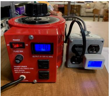
Meter on the autotransformer ("Variac<sup>™</sup>) is reading voltage to the radio or device/load connected. Hard to read here but it is 110 VAC.
