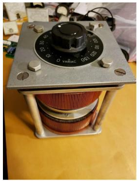
General Radio Dual W20G2 140-0-140 VAC Autotransformer Showing the two identical connection Showing the top panel with the voltage
