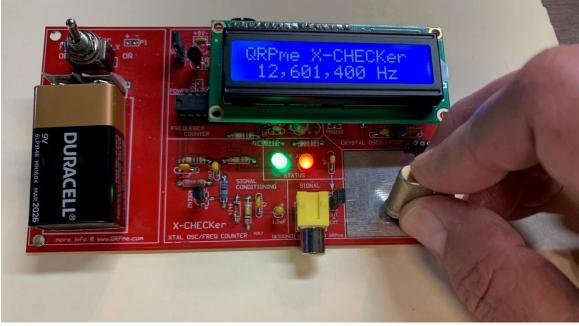
Checking a Crystal on the X-CHECKer
