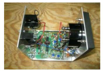
Once the circuit board and selector switches are completed the last step is to prepare the case for their installation. This involves installing and wiring the SO-239 connectors for RF in and out as well as the battery holder, power selector switch, and external power jack. Once this is all finished the meter will look like this inside:
