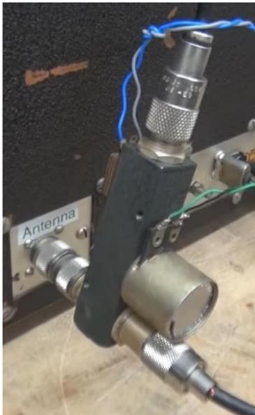
**Dow Key Antenna Switching Relay**
