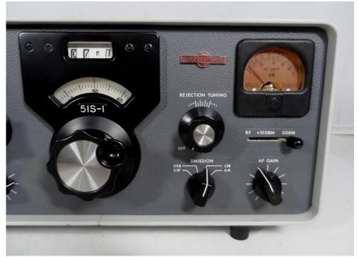
Collins 51S-1 Receiver REJECTION TUNING is between the Readout and the Signal Meter W9MXQ
