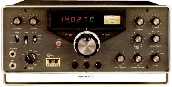
Below see the Omni D that was merely an Omni A with a digital readout.
