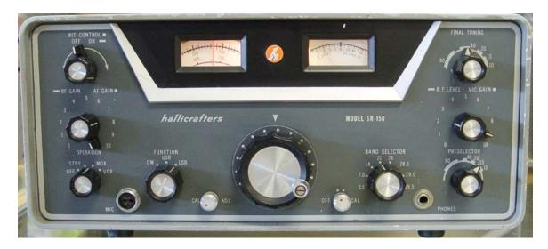
The front panel size of the SR-150 and the SR-400 were identical but complexity was increased in the later model. The addition of a very effective Noise Blanker, separate CW Filter, and Notch
