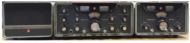
Left to Right PS-500A-AC AC Power Supply, SR-400 Cyclone II Transceiver, HA-20 DX Adapter
