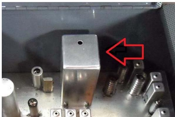
This large assembly in the back center of the radio chassis – reference the red arrow – is absent from HQ-170 and HQ-170A Receivers. It is present only in the HQ-170AC-VHF. Contained therein is a converter and pre-amplifier for 2-meters. The converter and pre-amplifier use the then new, and revolutionary, Nuvistor vacuum tube from RCA. Not much larger than a transistor, it was designed with its tiny internal elements to be effective at VHF and UHF frequencies.
