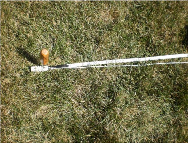
icepick through the hole of the end insulator, where the wire is attached, and push into the ground. Also fasten the end of your tape-measure to the awl. (Mine has a loop which I also pass the awl through.) Now lay out the wire alongside the length of the tape-measure, and find 16'-4 $\frac{3}{4}$ ". Right at that point, bend the wire 90 degrees. Measure 4-1/2" from the bend to-
