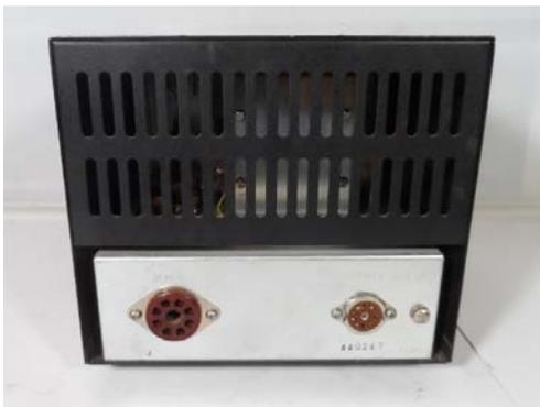
At the left, bottom picture, is a rear panel view of the Remote VFO. The small, 9-pin connector at the right is the interconnect to the TS-511S and carried VFO power, switching signals, and VFO RF to/from the transceiver. The eight pin “octal” socket is not generally use but contained connections to an internal relay that could be used for linear amplifier, receiver preamplifier, or other accessories.
