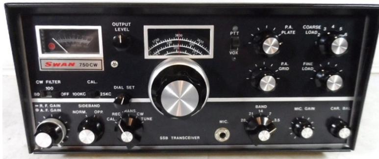
**Swan 750cw HF (80-10 Meter) SSB / CW Transceiver**
