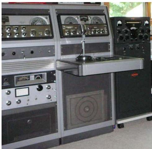
This is the Hallicrafters SR-500 Console. Note top left is the HT-30 Exciter. Top right is the SX-100 Receiver. Right below the HT-30 and a control panel is the HT-31 Amplifier. Note also the work shelf with the microphone. Behind screens are speakers that are not correct for the period.
