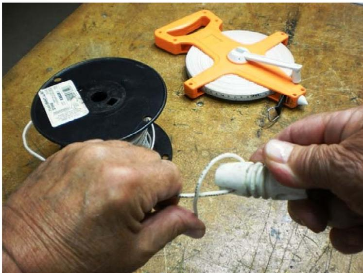
A 20 meter dipole is what I need to add to my arsenal of emergency/Field Day antennas. I already made the center insulator last month so all we need to do now is calculate the length of the two wires, fasten the end insulators, the center insulator, and solder. Using the formula, I'm going to divide 468 by 14.050 MHz which equals 33.3 feet for the total length of the antenna. (I chose the CW
