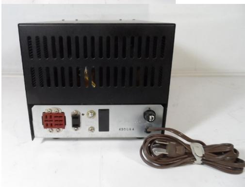
At the left, bottom picture, is a rear panel view of the power supply. You can see the “Cinch Jones” style 12-pin power connector for the transceiver, an AC socket for the 120 VAC fan. There is a final amplifier bias adjustment at the top center of the lower panel. There is a provision for the system AC fuse as well as a fixed AC power cord – a typical two-wire 120 VAC line cord of Kenwood at the time. Even much later Kenwood radios did not have a three-wire AC power cord.
