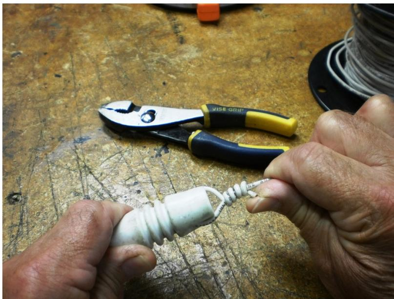
What I've found to be the easiest way to do this is to first attach an end insulator to the wire coming off of a spool or coil. You simply pass a few inches of the wire through the hole of the insulator and bend it around back to itself and closely wrap three or four turns. You might want to use a pliers to tighten the wrap. Whatever is left over can either be snipped off or wrapped further down. Now put an awl or
