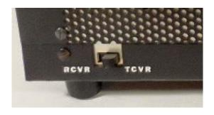
My Drake collection includes an early TR-4, a TR-4C, and a TR-4Cw-RIT. In every case, the switch pictured to the left is present on the left-lower-rear side of the cabinet. It switches the radio from using the Internal Transceiver (TCVR) or an External Receiver (RCVR).
