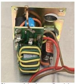
Mounting Side of IC-PS35 AC Power Closeup of the Access Panel that Supply with Access Panel to the right and standard power plug to the left. Of the IC-751A. Details of the Icom IC-PS35 Internal AC Power Supply W9MXQ Photos
