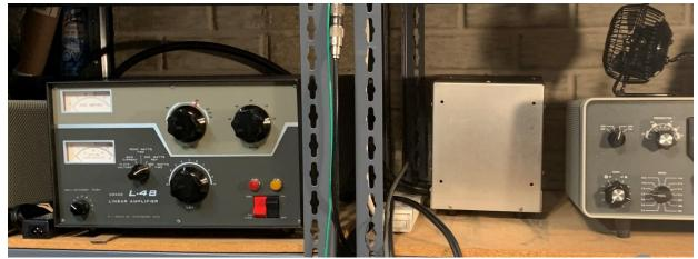
Right to left . . . Small Fan, sitting on top of a Collins 75S-3 Receiver, Drake L4-PS Power Supply Drake L-4B Linear Amplifier (Air Blows Right to Left, across L4-PS and L-4B)
