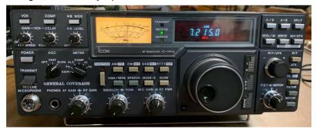
proved IC-751A version. The IC-751A came in an early version – showing the same Icom logo that dated from when Icom used the brand name "Inoue," and primarily made well respected VHF/UHF gear<sup>9</sup>. This relatively early all solid-state radio brought excellent receive audio, transmit audio, receiver AGC, and QRM Control as we have come to expect from modern radios – but remember that this was the 1980's. This radio basic design (original IC-751) is now over 40- years old.
