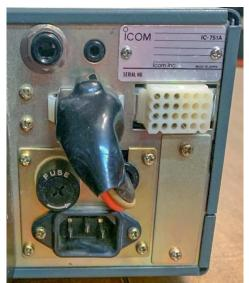
Icom IC-751A with the Optional IC-PS35 AC Power Supply Fitted W9MXQ Photo
