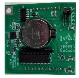
This is the Piexx Non-Volatile RAM Board. This retro-fit board plug in place of the Icom RAM board on the existing Logic Board. The CR-2032 battery is clearly in place in a removeable holder. It can be removed and replaced with no radio problems. The RAM chip (below the battery in this picture) is flash programmed and therefore permanent.
