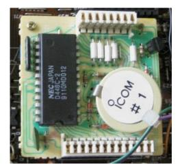
This is the RAM Board – as noted in the text, this is a board that plugs into the larger Logic Board. The round item that says "Icom #1" is the CR-2032 battery that is soldered in place. If removed, even for an instant, the radio becomes nothing more than an attractive collection of plastic, metal, and circuitry. The integrated circuit you see is the RAM chip.
