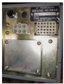
Icom IC-751A without the Optional IC-PS35 AC Power Supply Fitted KB9PRF Photo
